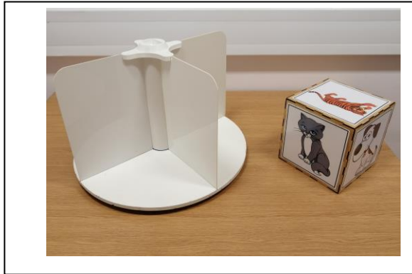
Figure 1. Turning table: the toy is placed on one side of the wall on the table so only Kaspar or the child can see the toy. Cube: there is a picture of an animal on each side. The child is asked to hold the cube so Kaspar can see a specific animal.
