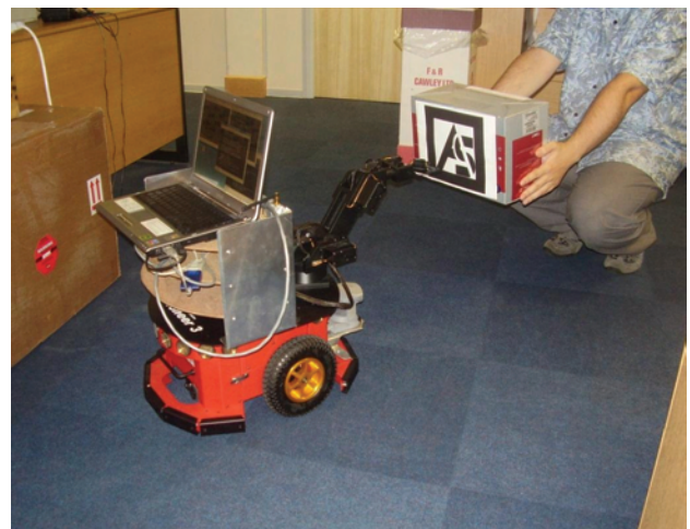
Fig. 1. The environment showing the Pioneer robot pointing to a patterned object. The robot is equipped with sonars, bump sensors, a pan/tilt camera and 5-DOF arm.
